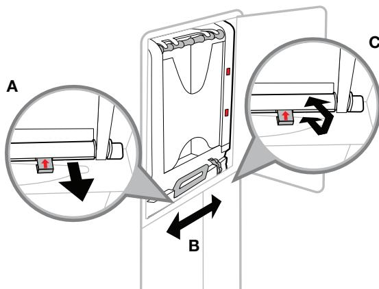
**A. Release the clips of the mounting bar. /**
